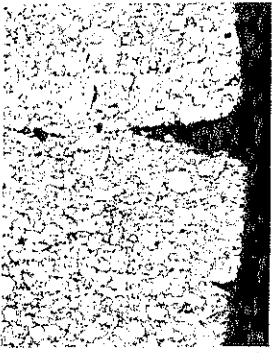
Figure 22.7 Photomicrograph of intergranular corrosion in a zinc die casting. Segregation of impurities to the grain boundaries produces microgalvanic corrosion cells ( \times 50 ).
